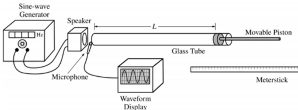
6. You are given the apparatus represented in the figure above. A glass tube is fitted with a movable piston that allows the indicated length  $L$  to be adjusted. A sine-wave generator with an adjustable frequency is connected to a speaker near the open end of the tube. The output of a microphone at the open end is connected to a waveform display. You are to use this apparatus to measure the speed of sound in air.
