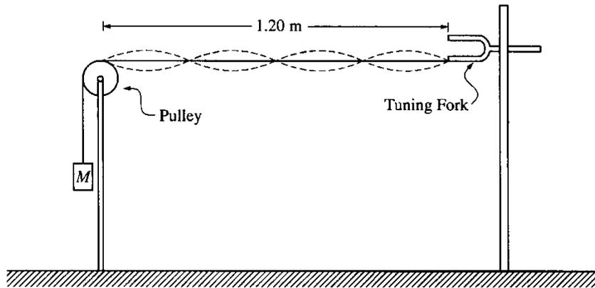
2. To demonstrate standing waves, one end of a string is attached to a tuning fork with frequency 120 Hz. The other end of the string passes over a pulley and is connected to a suspended mass  $M$  as shown in the figure above.
