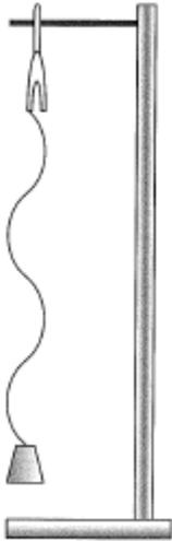
The same tuning fork is mounted vertically on a ring stand. A string of length 2m is attached to the tuning force and a mass  $m$  is hung on the end of the string. The tuning fork is activated, and a wave passes through the string (the size of the amplitude of the wave is exaggerated for clarity). Assume that the tension in the string does not affect the frequency of vibration of the tuning fork.
