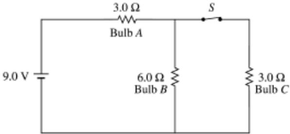
1. Lightbulbs of fixed resistance  $3.0 \Omega$  and  $6.0 \Omega$ , a  $9.0 \text{ V}$  battery, and a switch  $S$  are connected as shown in the schematic diagram above. The switch  $S$  is closed.
