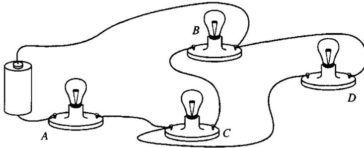
5. In the circuit shown above, A, B, C, and D are identical light bulbs. Assume that the battery maintains a constant potential difference between its terminals (i.e., the internal resistance of the battery is assumed to be negligible) and the resistance of each light bulb remains constant.
