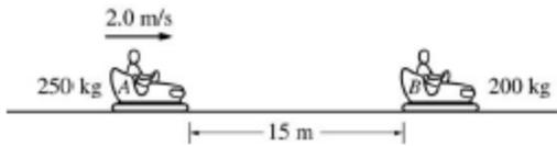
4. Several Students are riding in bumper cars at an amusement park. The combined mass of car A and its occupants is 250 kg. The combined mass of car B and its occupants is 200 kg. Car A is 15m away from car B and moving to the right at 2.0m/s, as shown, when the driver decides to bump into car B, which is at rest.
