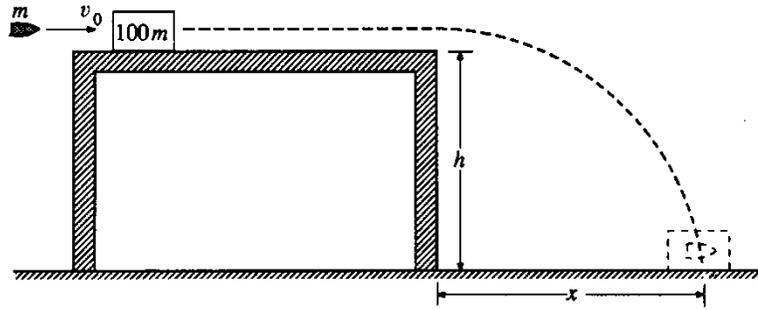
1. A bullet of mass  $m$  is moving horizontally with speed  $v_0$  when it hits a block of mass  $100m$  that is at rest on a horizontal frictionless table, as shown above. The surface of the table is a height  $h$  above the floor. After the impact the bullet and the block slide off the table and hit the floor a distance  $x$  from the edge of the table. Derive expressions for the following quantities in terms of  $m$ ,  $h$ ,  $v_0$ , and appropriate constants:
