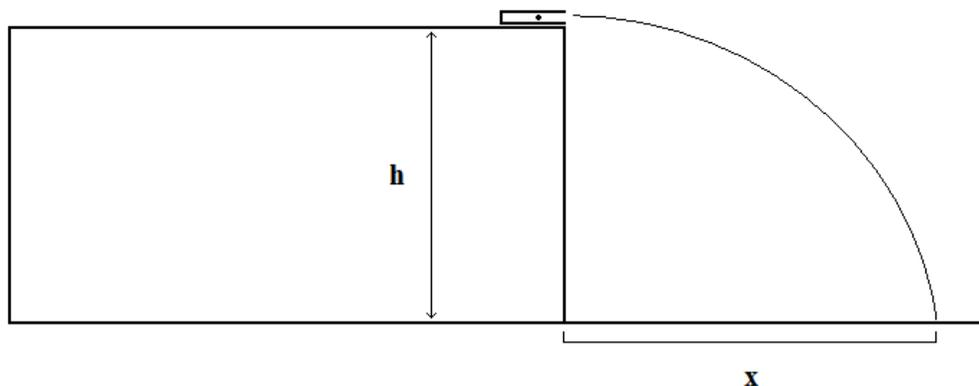
3c. Make a graph with horizontal flight distance (x) on the y-axis and spring compression distance (d) on the x-axis. If the regression line is linear, it suggests the spring constant of the spring remains constant at various compression distances.
