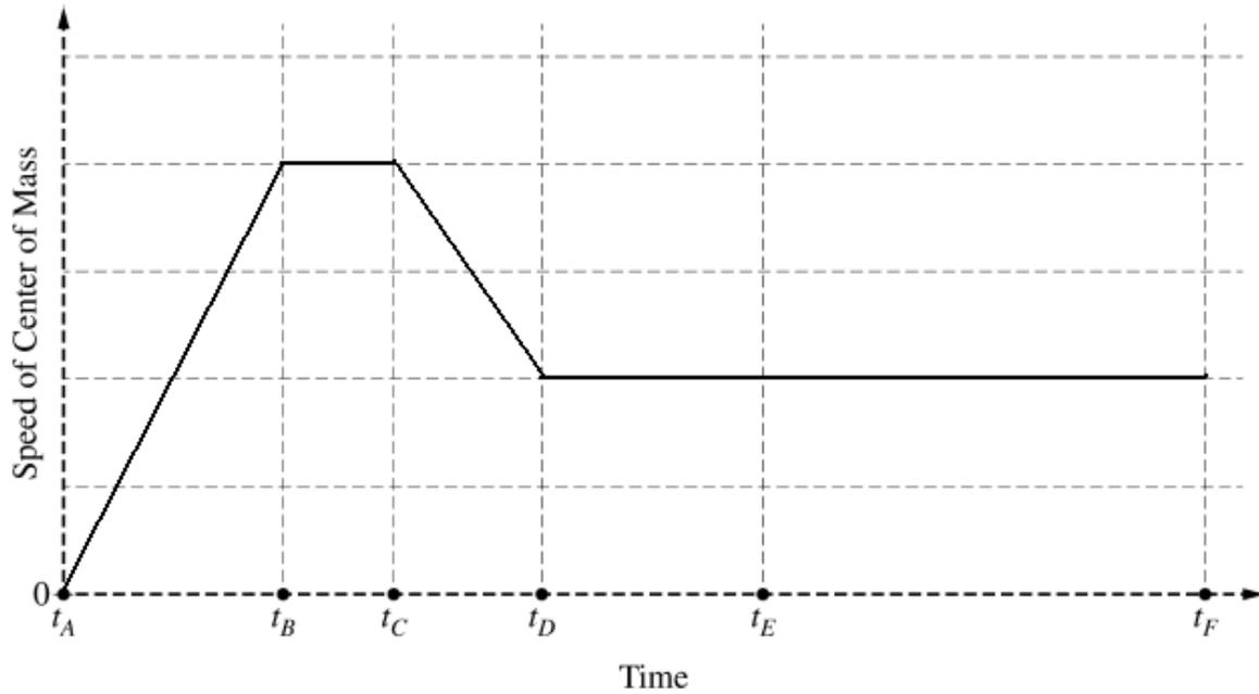
1b. From C to D only. Throughout the entire motion, the plunger, the normal force, and the force of gravity all apply a force through the center of mass. Therefore, as none of these forces apply a torque, they cause no change in angular momentum. From C to D, the force of friction does apply a clockwise torque which causes a clockwise change in angular momentum.
